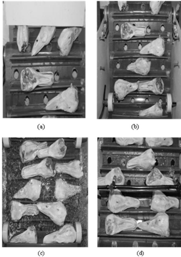
Fig. 6. Repetitious tests of prototype of (a) the separation of duck heads in storage box; (b) uniformity of duck heads; (c) the bubbling device in immersion box; (d) cleaning test in spray device
