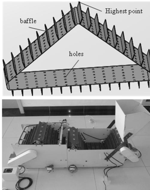
Fig. 5. Top-cleaning conveyor belt, right-actual structure of the prototype
