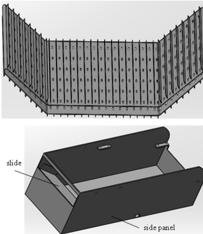
Fig. 3. Top-immersion conveyor belt, bottom-cleaning box
